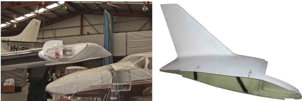
Figure 1: Hoerner tip geometry on the aircraft and original winglet prototype
