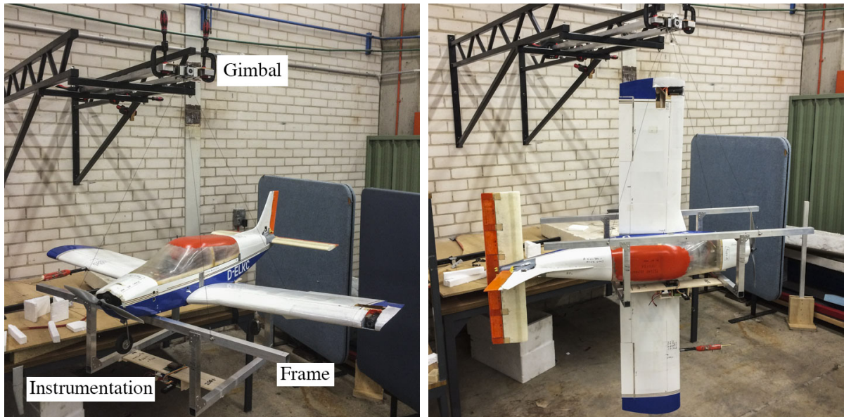
a) UAV on the support frame with data acquisition unit at the bottom of the frame
